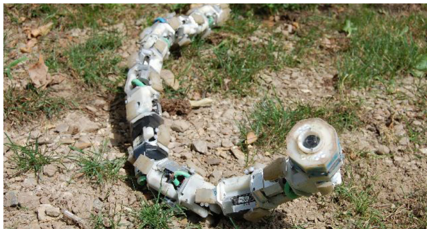
The Search Serpent Robot mimics the way a snake maneuvers. This high flexibility allows the robot to move through complex environments where people and conventional machinery cannot.
