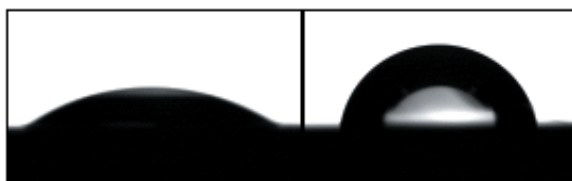
Figure 6: Graphical comparison of contact angle before and after the insulator surface is treated with a PFAPA SAM layer. PFAPA eliminates charge-trapping hydroxyl groups, leading to a more hydrophobic surface.
