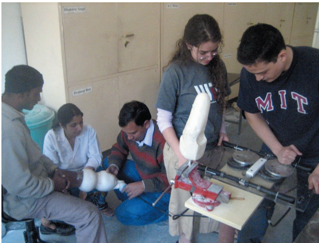
Figure 3: Two DWP team members test the Vac-Cast vacuum-forming device in a JFO clinic in Jaipur, India in January of 2008.
