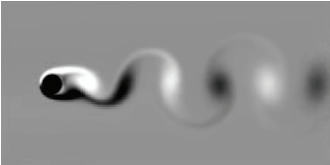
Figure 9: Simulator Vorticity Visualization Showing Well-Developed Vortex Street After About 50,000 Time Steps
