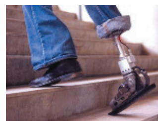
The robotic ankle-foot prosthesis developed at the MIT Media Lab by Professor Hugh Herr and researchers in the lab's biomechatronics research group.
